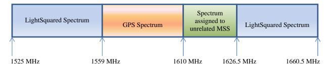
49. This illustration is not a complete depiction of all entities operating within the L-band and the RNSS-band. The illustration simply shows the main facts regarding the proximity of the LightSquared Spectrum and the GPS Spectrum and it will be referred to throughout the remainder of the Complaint to explain spectrum issues.
